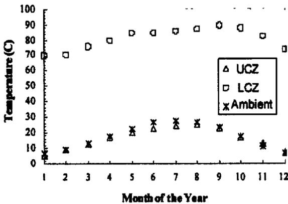
Fig. 3. Temperature development in the solar pond. UCZ, LCZ, upper and lower convective zones, respectively.
