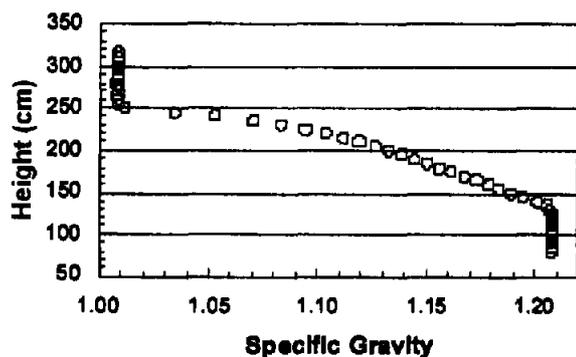
Fig. 1. Density profile of the El Paso solar pond on September 1, 1999.
