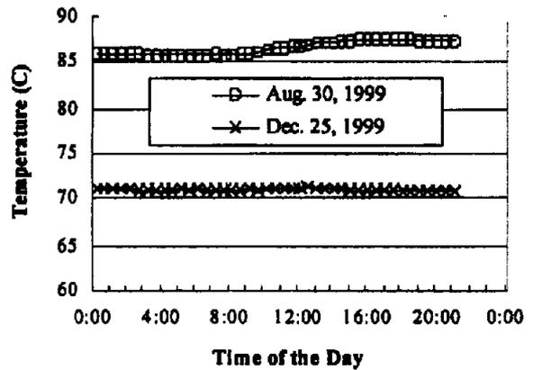
Fig. 4. Temperature variation in the LCZ of the El Paso solar pond during a day.
