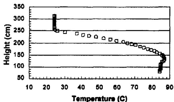
Fig. 2. Temperature profile of the El Paso solar pond (with heat extraction) on September 1, 1999.
